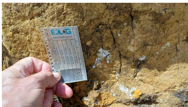
Fig.7. Stress fractures in a Marlstone block
