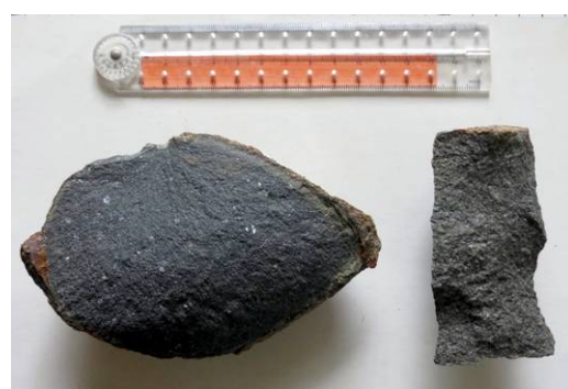
Fig.16. Porphyritic dyke rock (left) and Whin Sill (a quartz-dolerite, right)
