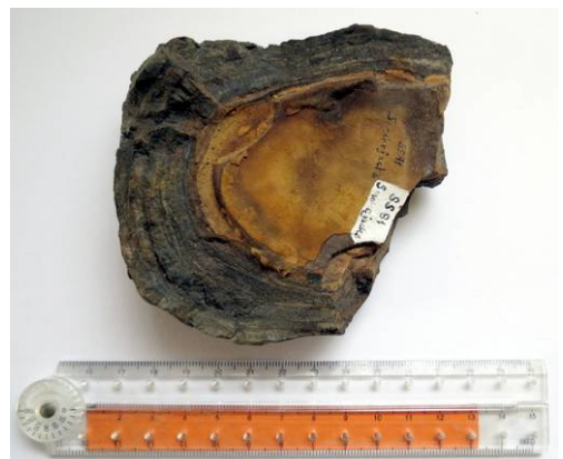
Fig. 12. Ironstone concretion with concentric layering: Weald Clay, Surrey
