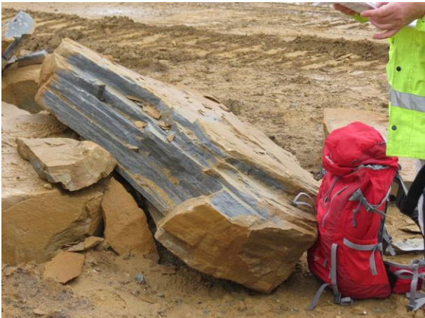
Fig. 3. Bedding running through a large 'dogger' concretion from the Collyweston Slate (cf. Fig. 10)
