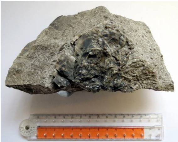
Fig. 18. Chert nodule (darker 'core') replacing limestone in colonial coral, Peak District
