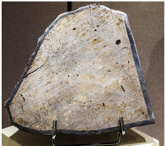
Fig. 11: Iron meteorite with Widmanstätten pattern, found Hammersley Range, Australia, © Raimond Spekking, Wikimedia Commons
