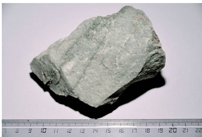
A specimen of metaquartzite showing its conchoidal-like fracture and granular texture.
