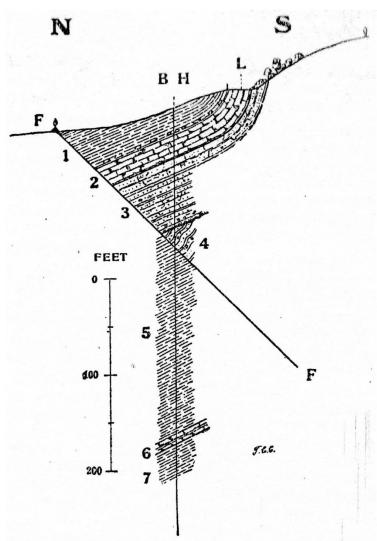
FIG. 2.—Vertical section, in a north and south plane, of the upper part of the Folly Farm Borehole, Presteign. L, lane; BH, borehole; F-F, overthrust fault; 1, 5, and 7, Wenlock Shales; 2, Woolhope Limestone and Shales; 3, Upper Llandovery Sandstone; 4, supposed Archæan (Longmyndian); 6, 12 ft. limestone-band.
